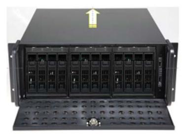
Once the screws removed, push the top cover to remove from the chassis.
