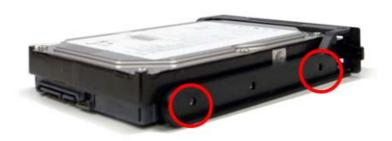
Once align, you can fasten the screws on both side of the tray to fix the HDD.
