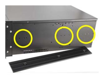
Upon removing the side bar, you will find several screw holes for you to install the server rail.
