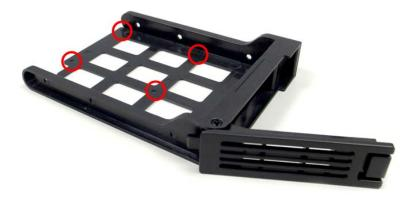
To install a 2.5" HDD, please make sure that the 2.5" HDD is align with the screw holes on the tray
