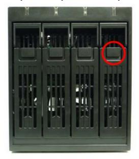
Each HDD Tray has a press button for releasing the hinge. To remove the HDD Tray; first press the button (red circle).
