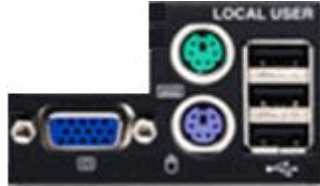
Figure 91: Local User Panel on Dominion KX II
