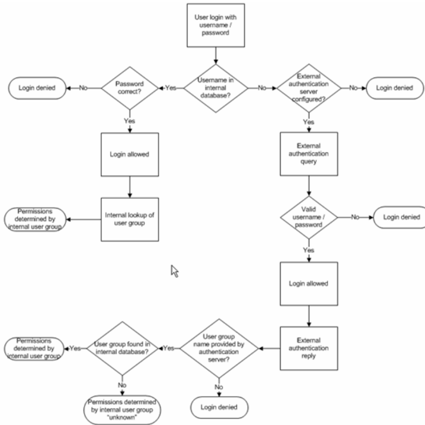
Figure 10: Authentication/Authorization Flow Diagram
