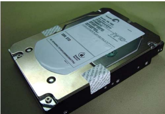
Figure 19. Example of FIPS tamper evidence labels.
