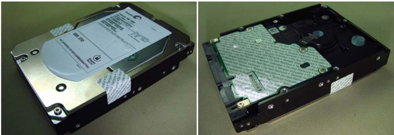
Figure 13. Example of FIPS tamper evidence labels.
