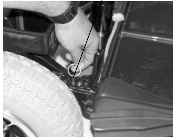
FIGURE 19. BALL DETENT PIN
