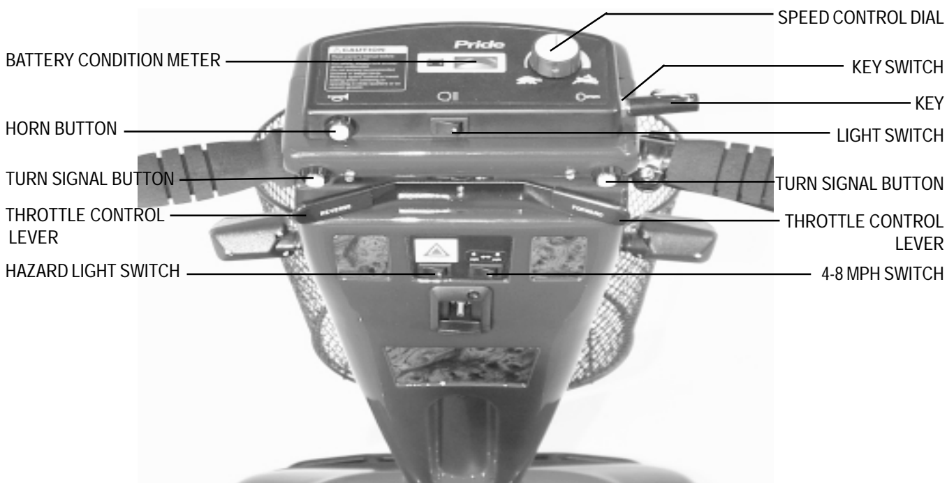
FIGURE 6. CONTROL CONSOLE ASSEMBLY
