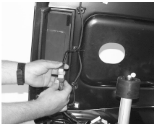
FIGURE 14. REAR LIGHTING HARNESS
