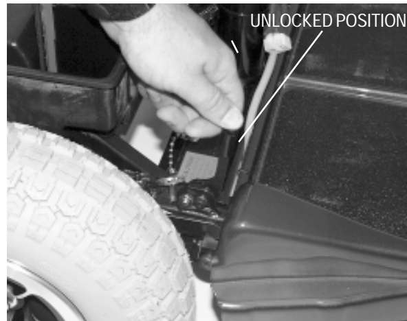
FIGURE 20. FRAME LOCK LEVER
