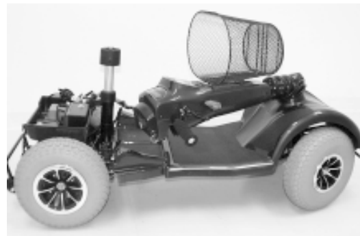
FIGURE 9. TILLER FULLY LOWERED
