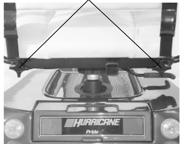
FIGURE 12. ARMREST WIDTH ADJUSTMENT
