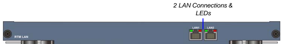
Figure 1-13 RMX 4000 RTM LAN Rear Panel Layout
