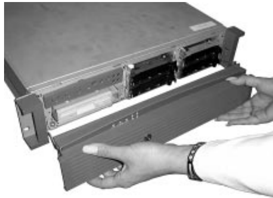
Figure 6. Opening the Bezel
