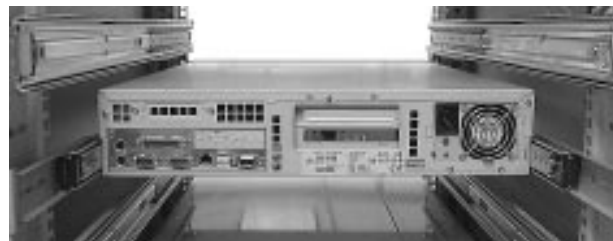
Figure 33. Chassis Mounted into the Rack
