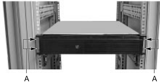
Figure 21. Mounting the Front Brackets to the Cabinet Chassis
