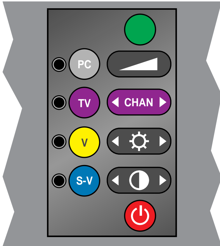
Figure 14: The keys on the touch panel on the KODAK DP1050 ULTRA projector
