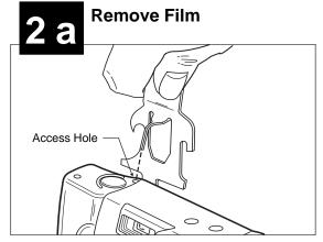
• Insert the punch end of the opening tool into the Access Hole.
