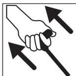
**12****Move the Choke to the OPEN Position**
