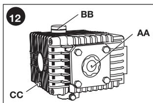
2. Place a container under the oil drain plug (CC).
