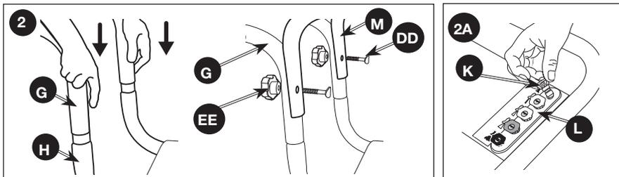
5. Remove colored quick connect nozzles (K) from plastic bag and insert them into correct grommet on the nozzle holder (L). **NOTE:** Nozzles are color coded to match colored nozzles on panel.
