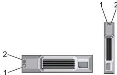
Figure 5. SCv300 and SCv320 Expansion Enclosure Drive Indicators
