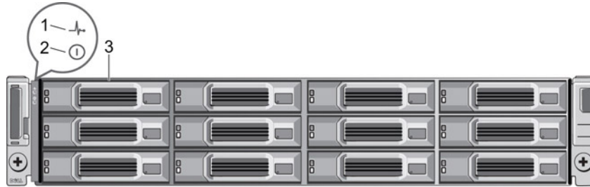
Figure 16. SC100 Front-Panel Features and Indicators
