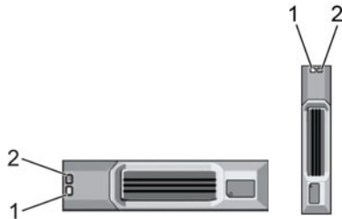
Figure 20. SC100/SC120 Drive Indicators
