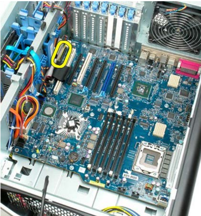
13. Disconnect the I/O panel cable.
