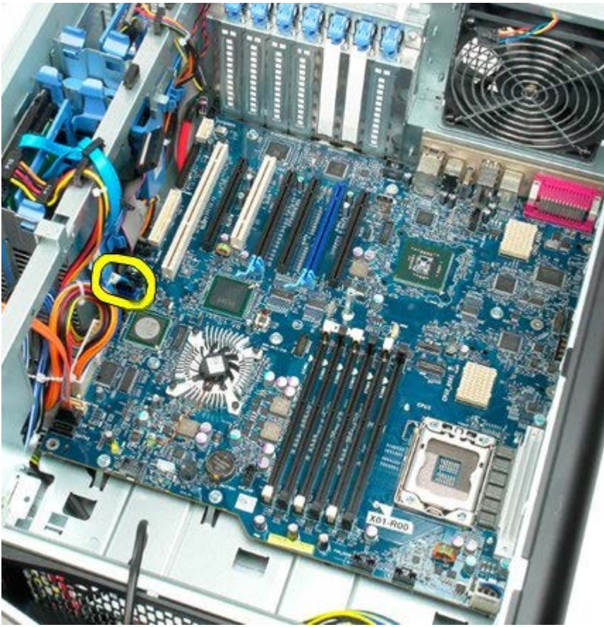
16. Disconnect the power supply cable.
