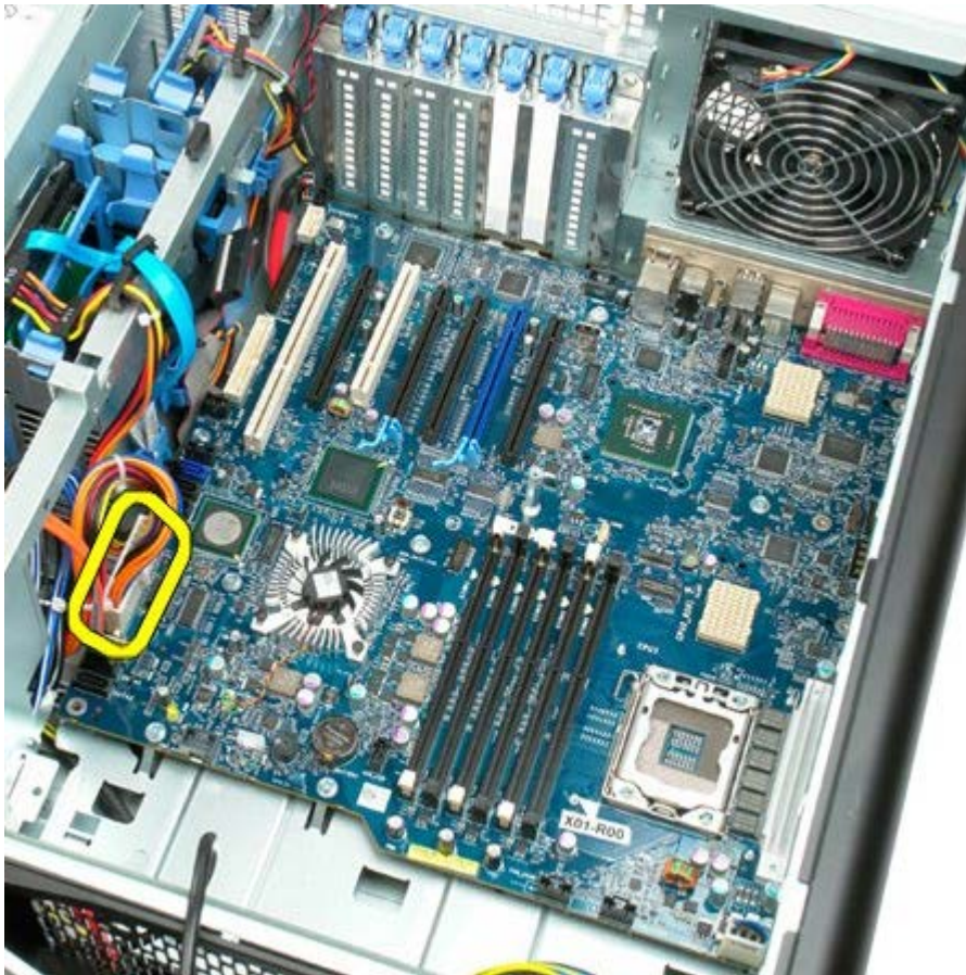
17. Disconnect the optical drive data cable.
