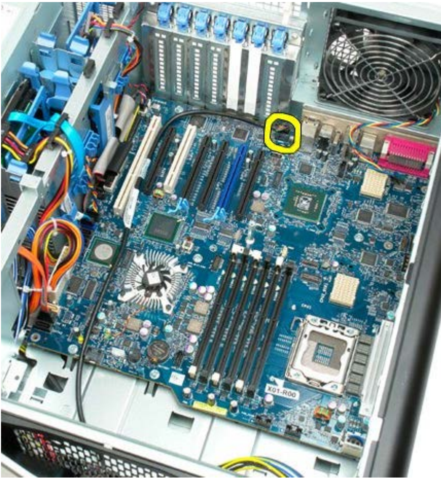
10. Disconnect the intrusion switch cable.
