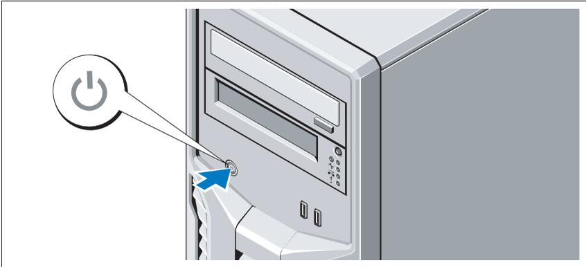
Press the power button on the system. The power indicator should light.
