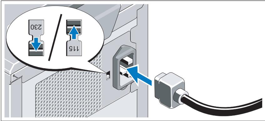
**CAUTION:** Be sure to set the voltage selection switch on the power supply for the voltage that most closely matches the AC power available at your location.
