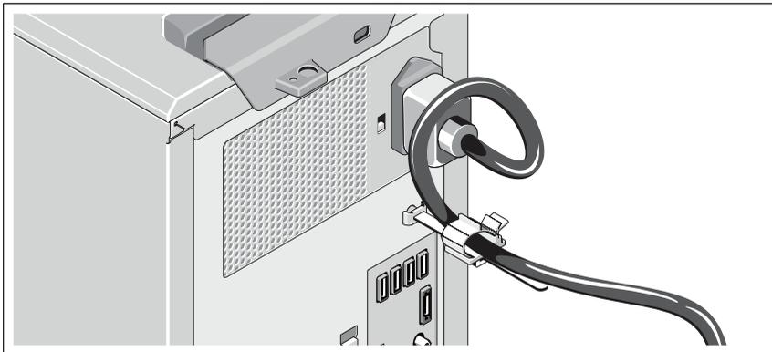
Bend the system power cable into a loop as shown in the illustration and attach to the cable clasp.
