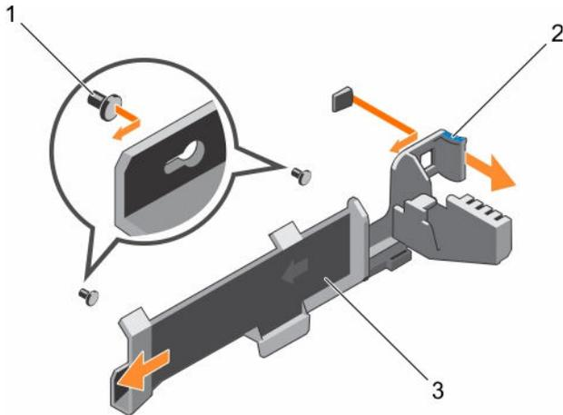
**Figure 29. Removing the cable retention bracket**
