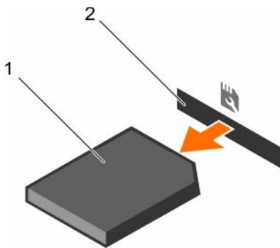
**Figure 78. Removing the SD vFlash media card**
