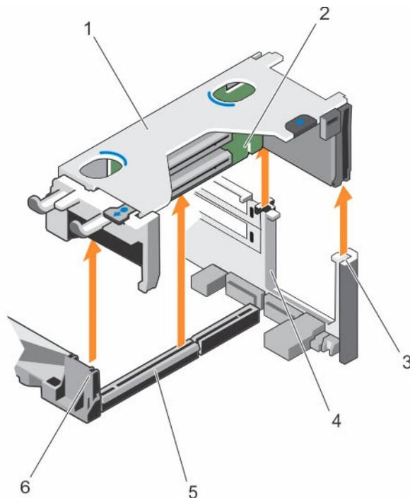
Figure 39. Removing the expansion card riser 1
