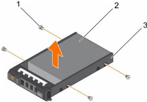
Figure 71. Removing a hard drive into a hard drive carrier
