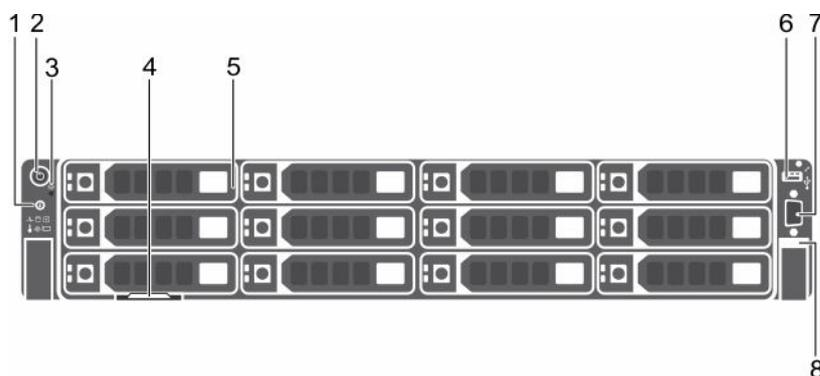
**Figure 1. Dell DR4300 system front panel features and indicators**
