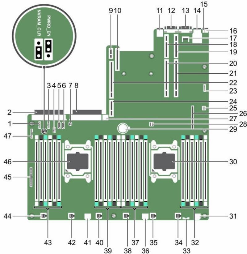
Figure 86. System board jumpers and connectors
