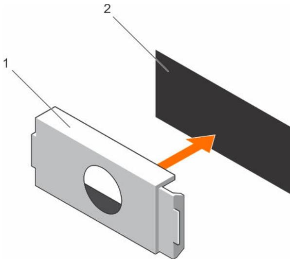
Figure 59. Installing the PSU blank
