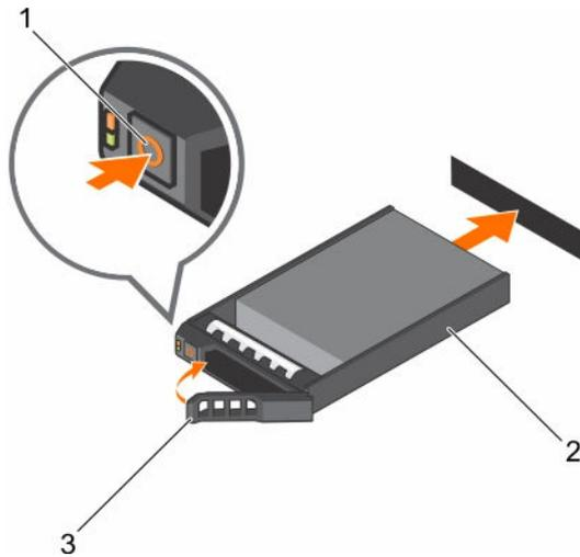
**Figure 70. Installing a hot-swappable hard drive or SSD**
