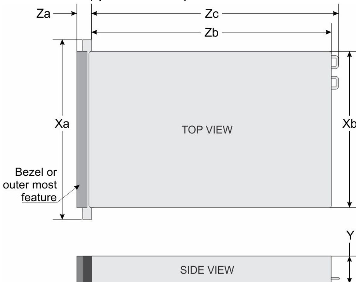
Figure 8. Chassis dimensions of your Dell DR4300 system
