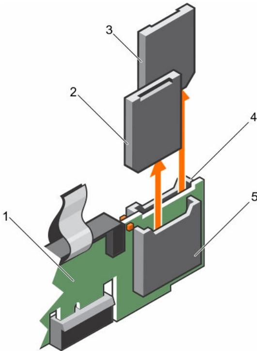
Figure 49. Removing an internal SD card
