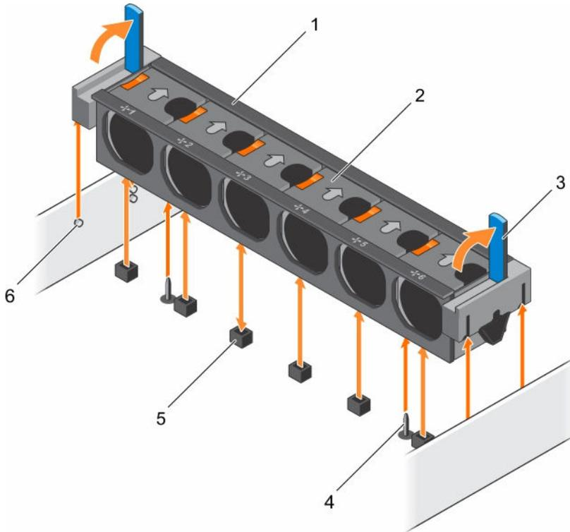
**Figure 15. Removing the cooling fan assembly**
