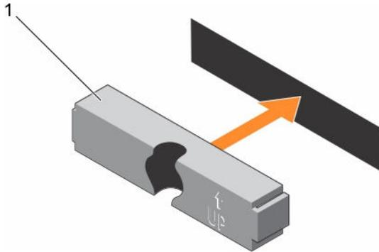
Figure 66. Installing a 2.5 inch hard drive blank (rear)
