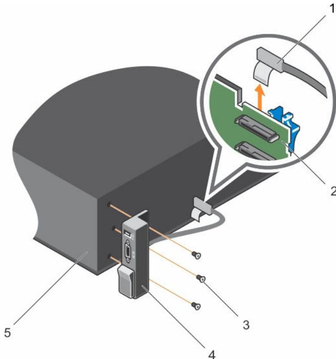
**Figure 84. Removing the I/O panel**
