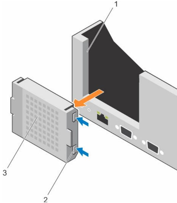
**Figure 37. Removing the riser 1 blank**
