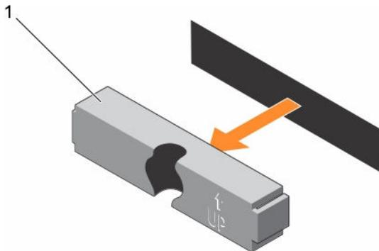
**Figure 65. Removing and installing a 2.5 inch hard drive blank (rear)**
