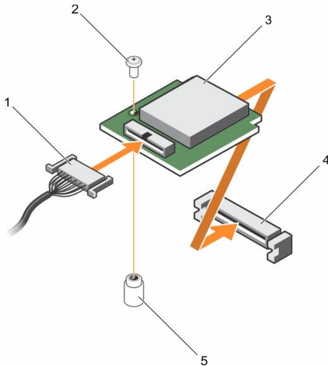
**Figure 81. Installing the vFlash media unit**
