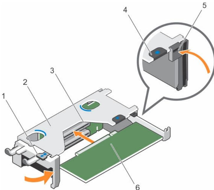
**Figure 36. Installing an expansion card into the expansion card riser 1**
