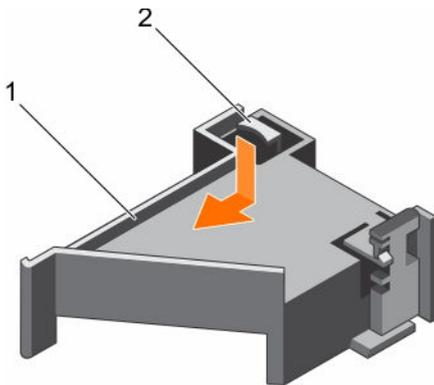
Figure 26. Installing the PCIe card holder
