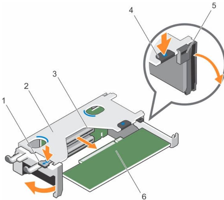
**Figure 35. Removing an expansion card from expansion card riser 1**
