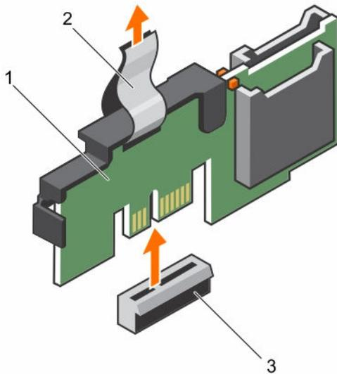
**Figure 51. Removing the internal dual SD module (IDSDM)**
