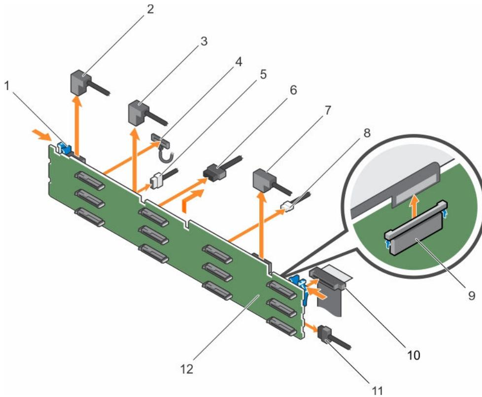
**Figure 73. Removing the 3.5 inch (x12) SAS/SATA backplane**
