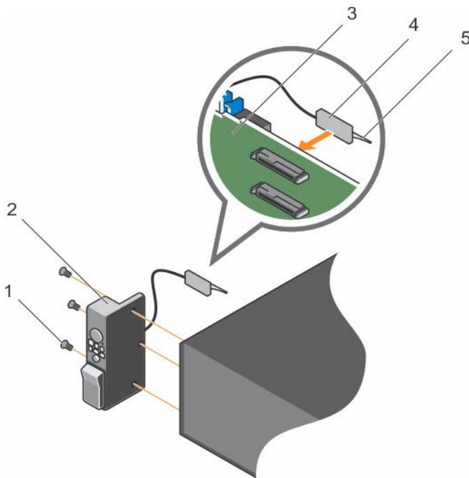
**Figure 83. Installing the control panel**
