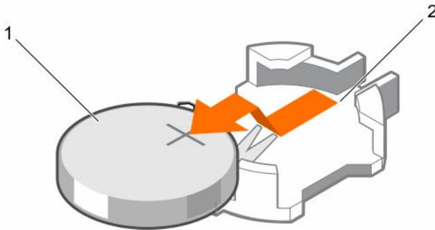
**Figure 56. Removing the system battery**
