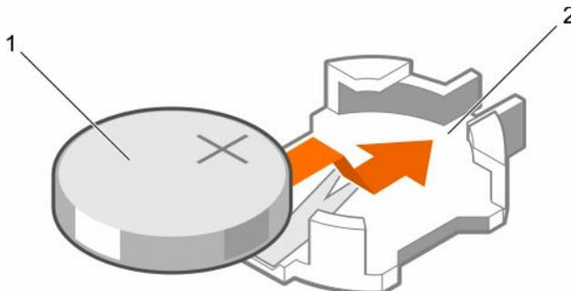
**Figure 57. Installing the system battery**
