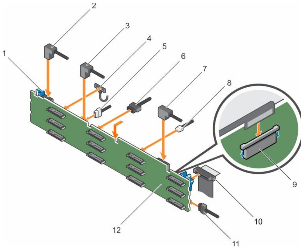
**Figure 75. Installing the 3.5 inch (x12) SAS/SATA backplane**
