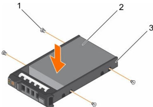
Figure 72. Installing a hard drive into a hard drive carrier
