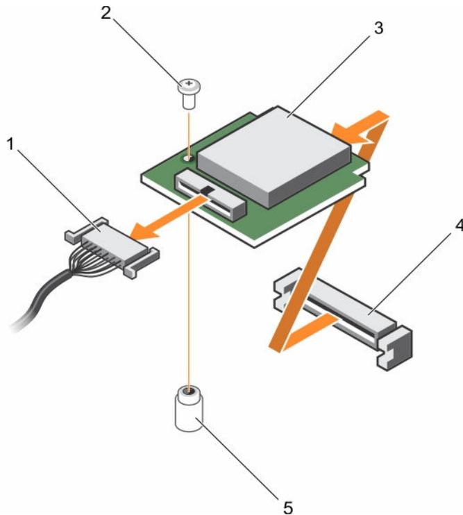
Figure 80. Removing the vFlash media unit
