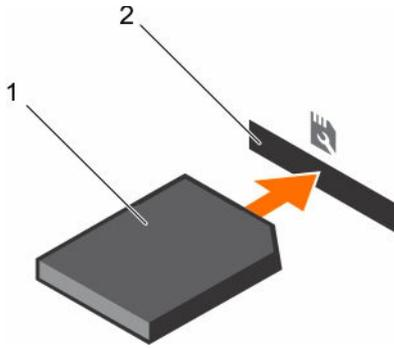
**Figure 79. Installing the SD vFlash media card**
