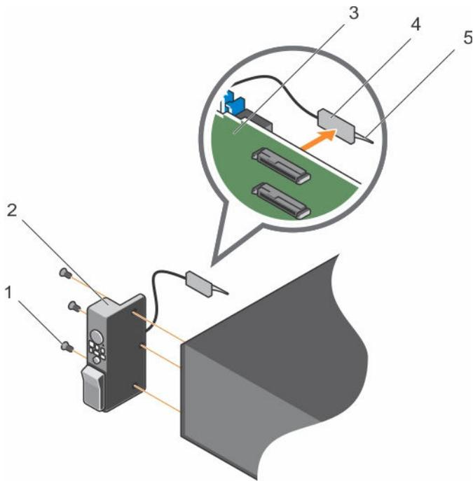
**Figure 82. Removing the control panel**
