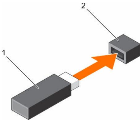
Figure 55. Installing the internal USB memory key
