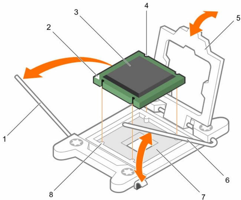
**Figure 22. Removing a processor**
