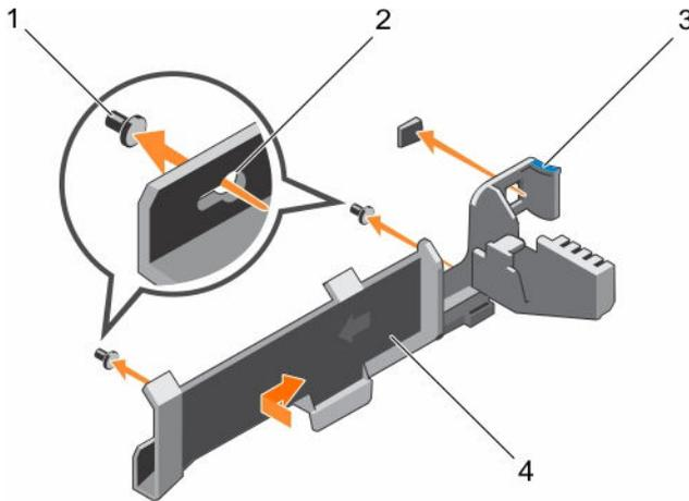
**Figure 30. Installing the cable retention bracket**
