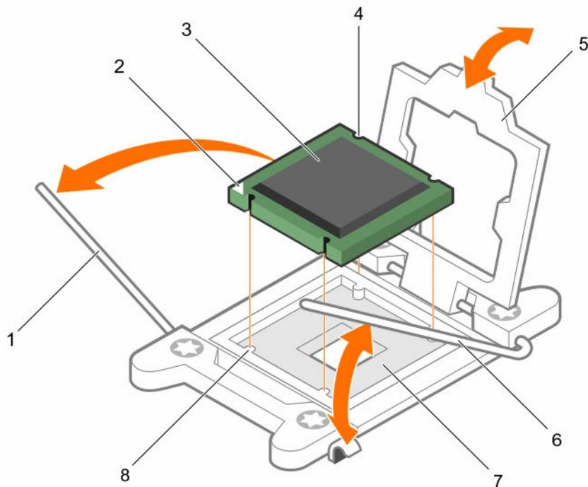
**Figure 23. Installing a processor**
