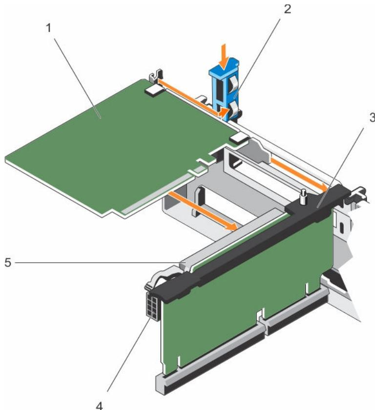
**Figure 34. Installing an expansion card into the expansion card riser 2 or 3**
