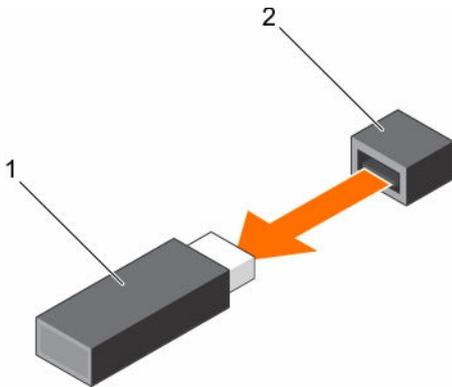
Figure 54. Removing the internal USB memory key
