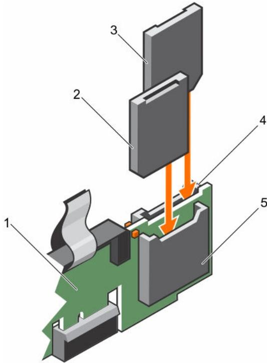
Figure 50. Installing an internal SD card
