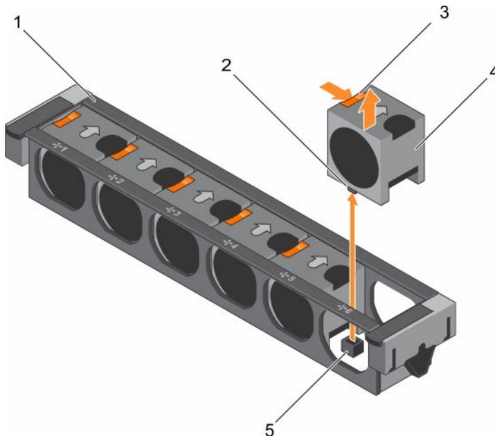
**Figure 14. Removing a cooling fan**
