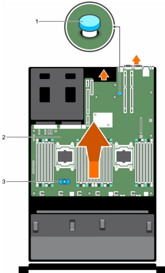
**Figure 63. Installing the system board**
