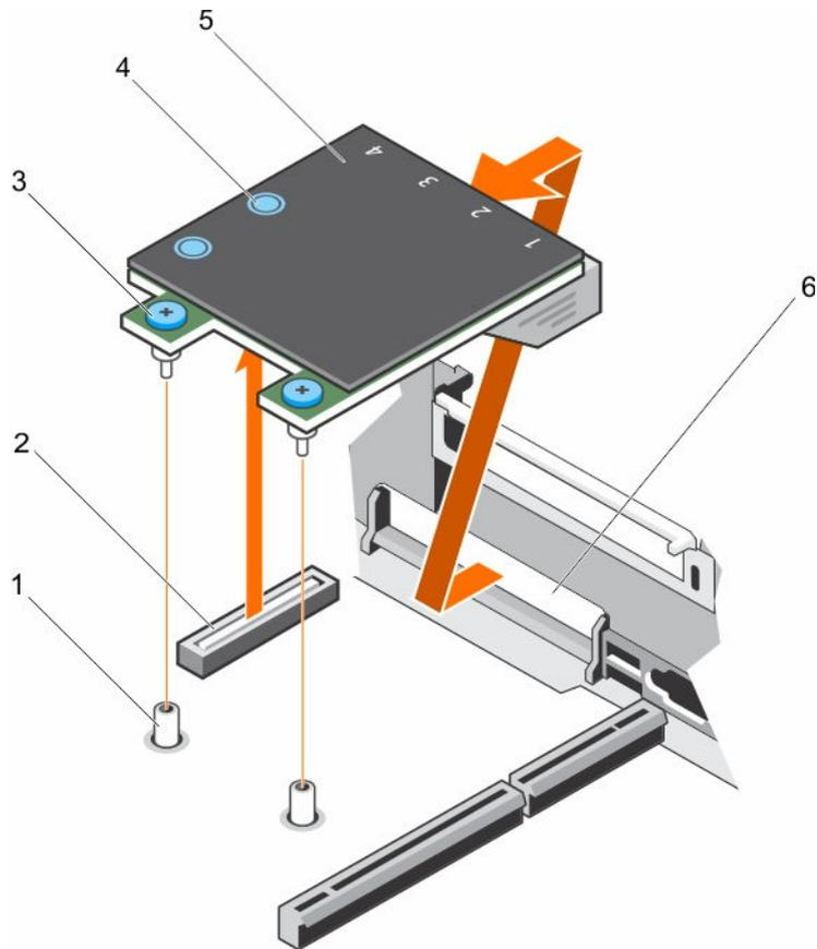
**Figure 52. Removing the NDC**
