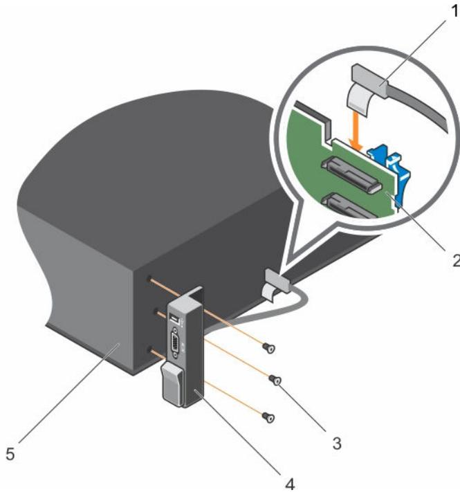
**Figure 85. Installing the I/O panel**
