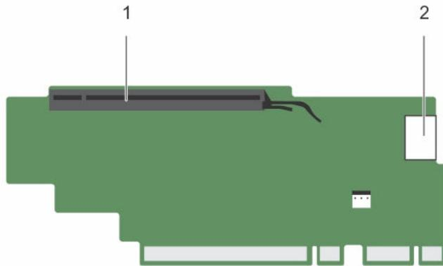
**Figure 45. Identifying connectors on the expansion card riser 3 (alternate)**
