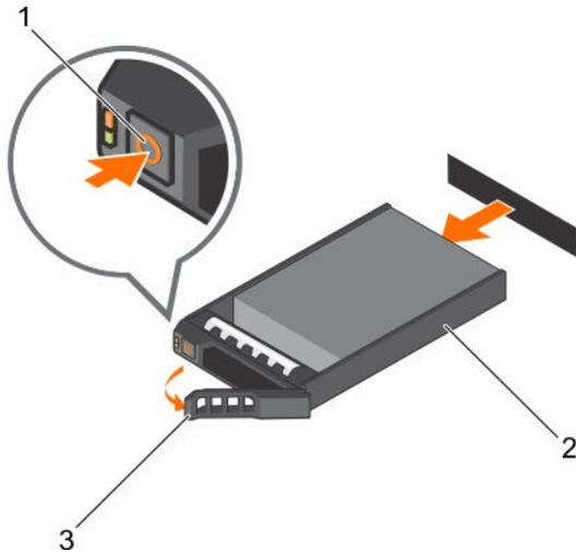
**Figure 69. Removing a hot swappable hard drive or SSD**
