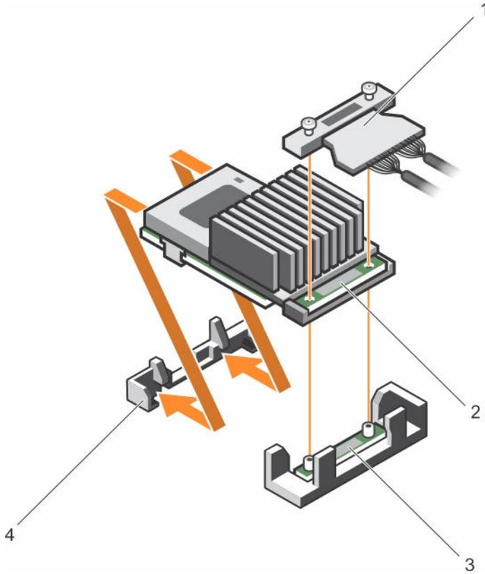
**Figure 32. Installing the integrated storage controller card**
