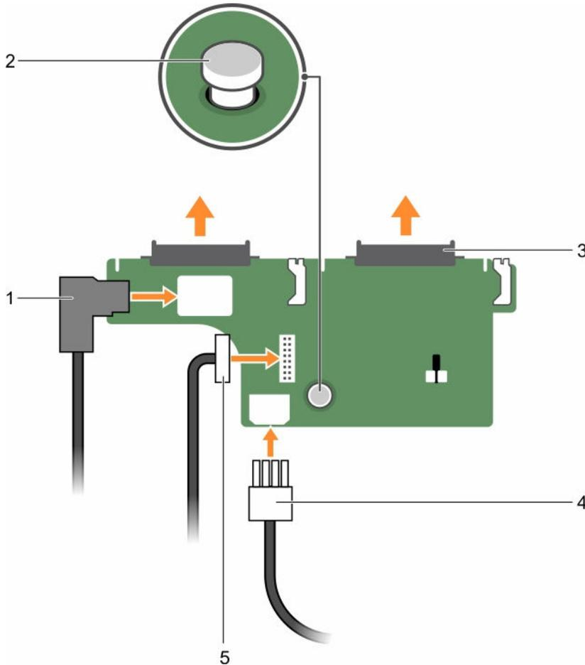
**Figure 77. Installing the optional 2.5 inch (x2) hard drive backplane**
