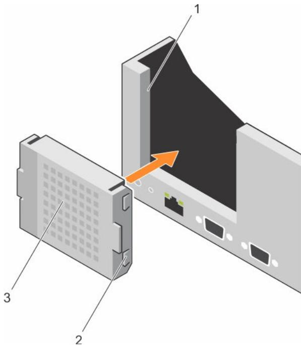
Figure 38. Installing the riser 1 blank
