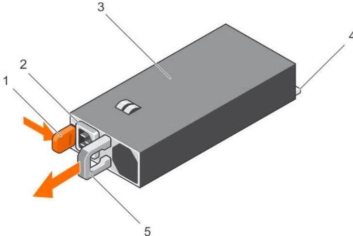
**Figure 60. Removing an AC PSU**
