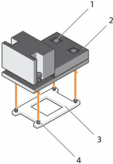
**Figure 20. Removing a heat sink**
