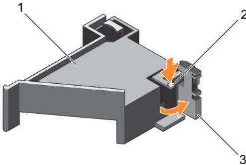
**Figure 27. Opening the PCIe card holder latch**
