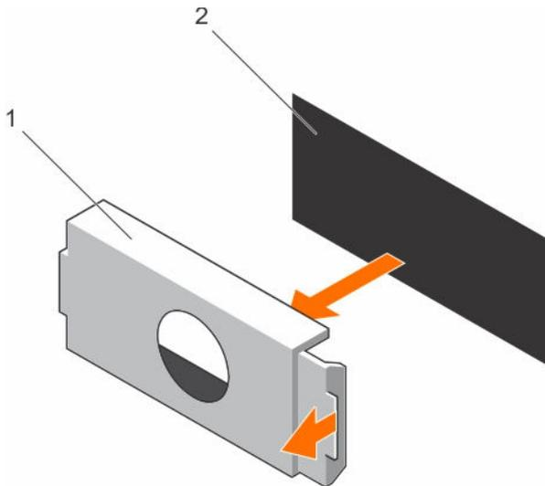
Figure 58. Removing the PSU blank
