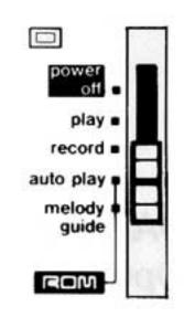
3 Select one of the tunes on the ROM pack by pressing the corresponding key on the keyboard. Pressing any other key on the keyboard will automatically select the first tune on the ROM pack.
