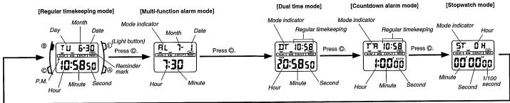
(Reversion to regular timekeeping) The watch reverts to regular timekeeping mode when © button is pressed after operation, regardless of mode
