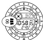
**Answer:** The face of this watch is marked with values that increase in a counterclockwise direction. These values represent degrees. When you take a direction reading, you can use these values to find out how many degrees the 12 o'clock position of this watch differs from magnetic north.
