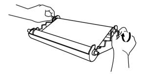
f 8 Turn the cartridge over and re-install it into the machine: Insert the recessed riangleq first and place the cartridge into its four holders.
