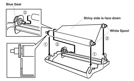
7 Turn the upper right white spool *clockwise* to tighten the ribbon, as shown.
