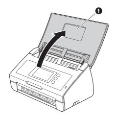
Pull the Output Tray out of the machine ①, and then unfold the Document Stopper ②.
