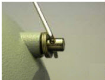
Figure 2.10: Replace 3 washers on shaft
