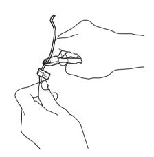
6. Press the connector onto the contact pin, marked A, on the charging station.
