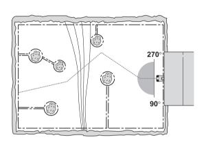
Area: 0.15 acre (600 m²). L-shaped garden with the charging station placed in the large open area. No guide wire is necessary.
