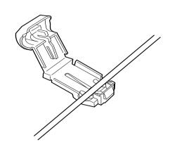
4. Press the connector together using a pair of pliers. Press until you hear a click.
