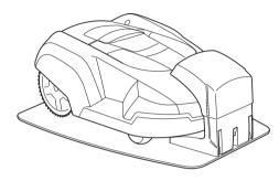
Good contact is made when both the charging strips on the mower touch the centre of the contact strips on the charging station.
