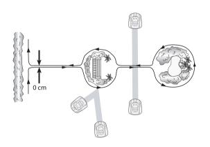
Obstacles that can withstand a collision, for example, trees or bushes higher than 6" (15 cm), do not need to be demarcated by the boundary wire. Automower® will turn when it collides with this type of obstacle.
