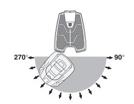
When Automower® body hits an obstacle, the mower reverses and selects a new direction.
