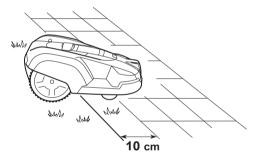
When the working area is divided by a flat slab path that is level with the lawn, it is possible to allow Automower® to run over the path. It can be an advantage to lay the boundary wire under the slabs. The boundary wire can also be laid in the joint between the slabs.
