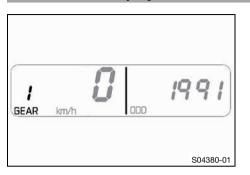
The gear display shows the engaged gear.
