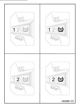
The combination switch displays the current riding mode and traction control setting.
