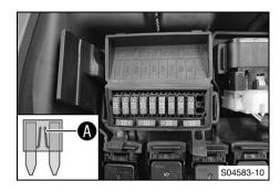
Remove the faulty fuse.
