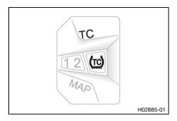
The motorcycle traction control (<u>cornering MTC</u>) lowers the engine torque in case of loss of traction in the rear wheel. Depending on the riding mode, different amounts of slip are allowed when the traction control is activated.
