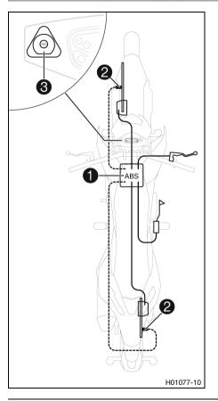
The ABS module ①, consisting of a hydraulic unit, an ABS control unit, and a return pump, is located under the seat. One wheel speed sensor ② is located in each case on the front and the rear wheel.
