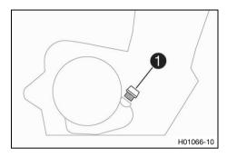
Mount and tighten filler plug 1 together with the O-ring.
