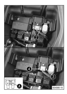
Remove a defective main fuse 3 with needle nose pliers.
